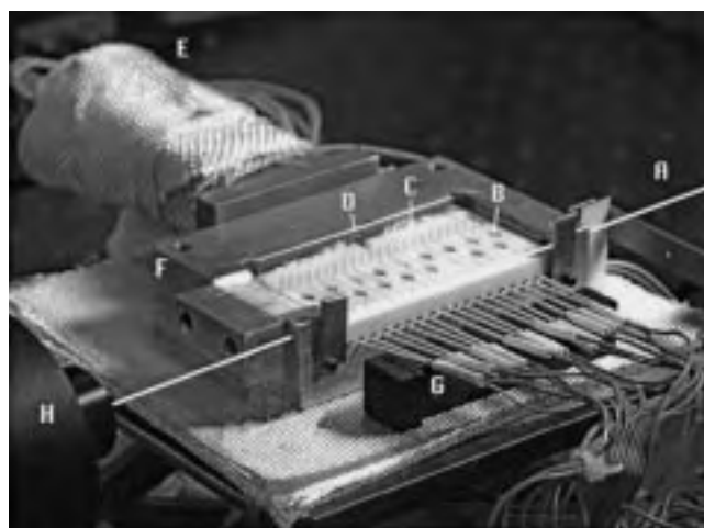
Figure 6. Array microreactor equipped with REMPI-screening components. A) Laser beam, B) catalyst pellets in wells, C) flow distribution baffles, D) feed-gas line, E) feed-gas preheater, F) metal heating block, G) electrodes, H) laser-power meter.
